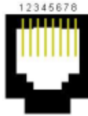
Figure 2-14 10/100 Ethernet Port Pin order
